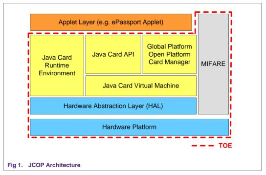
The Java Card virtual machine (JCVM) is responsible for ensuring language-level security; the JCRE provides additional security features for Java Card technology-enabled devices.
